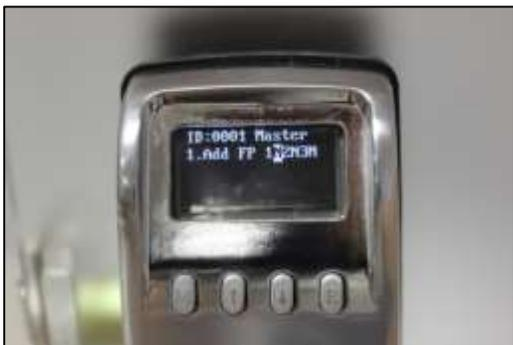
5) "Add FP" is displayed along with "1N2N3N". "1N" is highlighted. Place finger on the sensor. Press **M**.
