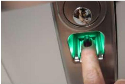
3) If fingerprint verification is successful, a single short beep will be heard, the green LED will flash and the RTS will unlock. It will remain unlocked for approximately four seconds.
