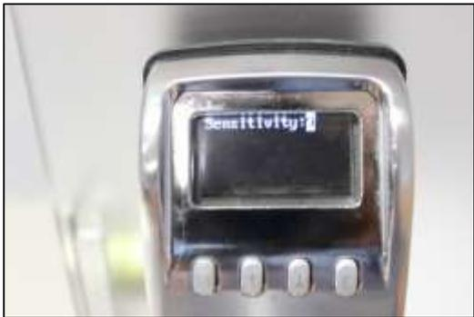
2) Use the Up/Down arrows to scroll through the sensitivity levels until the desired level is reached. Press **M**.
