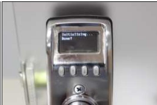
"Initializing Done!" is shown when the reset is complete.
