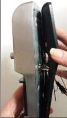
1) Attach the rubber gasket to the back of the outdoor unit. Repeat this step for inside unit.
