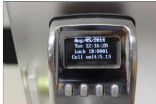
5) Press **M** on the inner keypad of your RTS to initialize the lock and display the current battery voltage.
