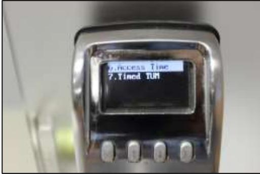
1) In the Lock setup menu, scroll to Option 6 "Access Time". Press **M**.
