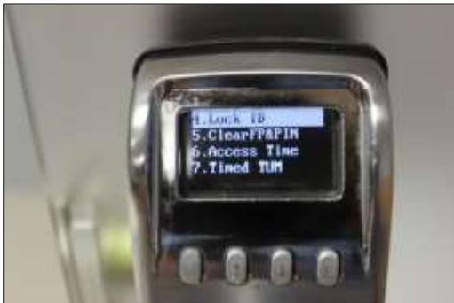
1) In the Lock Setup menu, scroll down to Option 4 "Lock ID". Press **M**.
