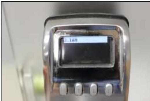
4) **1&N** - All enrolled users can use either the **1:1** or **1:N** method to unlock the door. This is the factory default setting.
