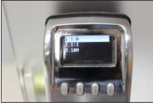
2) **1:N** - When this is chosen, all users enrolled at this lock only need to match their enrolled Fingerprint OR PIN Code to unlock the door.
