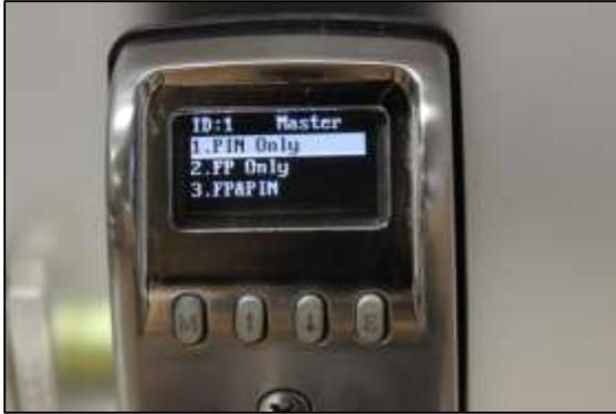
This menu will be displayed. It allows deletion of "PIN Only", "FP Only", or both "FP&PIN".
