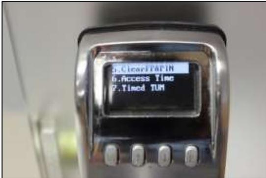
1) In the Lock setup menu, scroll down to Option 5 "Clear FP & PIN" Press **M**.
