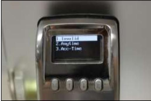
1) **Invalid** -This can also be called lock down mode. When this is enabled, only Administrators for the specific lock will have access to unlock the door.
