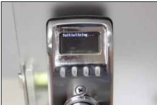
"Initializing" is shown while the lock is being reset.
