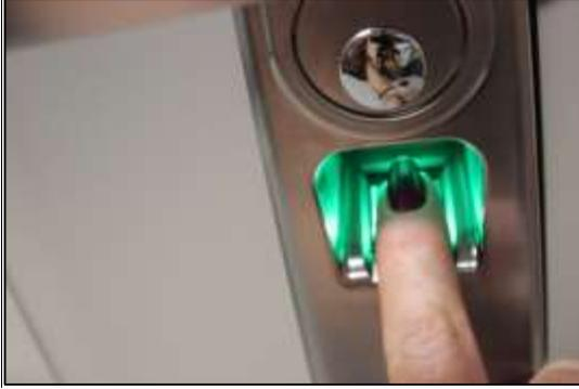
3) After the fingerprint sensor illuminates, place a finger on the sensor window.
