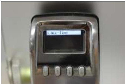
3) **Acc-Time** (Access Time) - This mode allows for timed access to the lock to be created for a specific date range, days of the week and time frame within the days of the week.
