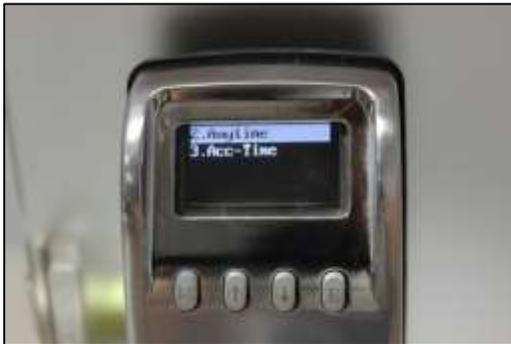
2) **Anytime** - When this is chosen, the lock allows all enrolled Users to unlock the door. The exception to this is if specific Timed Access is set up for individual Users (see Section 2: User Edit).
