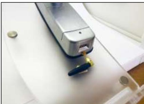
1) Take the antenna out of bag "E" and remove red plastic cover. Then screw the antenna on the bottom of the inside unit.
