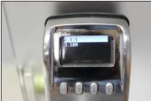
3) **1:1** - When this is chosen, all users enrolled at this lock must enter their User ID and verify their enrolled Fingerprint or PIN Code to unlock the door.
