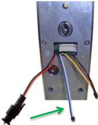
Normally open wires are the blue and white wires. These can be connected to a relay device.
