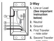
**IMPORTANT:** For 3-Way applications, note that one of the screw terminals from the old switch being removed will usually be a different color (Black) or labeled Common. Tag that wire with electrical tape and identify as the common (Line or Load) in both the dimmer wall box and remote wall box.
