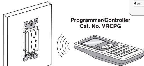
**NOTE:** Programmer/Controller must be in close proximity to receptacle when including in the network.
