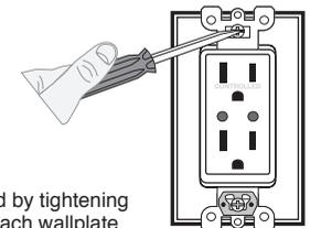
Installation may now be completed by tightening mounting screws into wall box. Attach wallplate.
