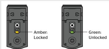
**B** Use your key to lock and unlock your door, and verify that the Status LED is communicating correctly.
