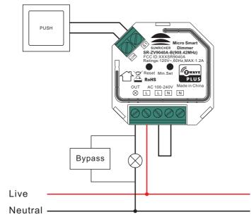
NOTE: Switch connected to the S1 terminal activates the basic functionality of the dimmer (turning the light on/off, dimming) and starts the inclusion/exclusion mode (Add/Remove).
