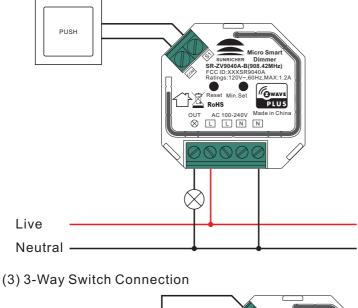
activates the basic functionality of the dimmer (turning the light on/off, dimming) and starts the inclusion/exclusion mode (Add/Remove).
