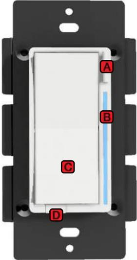
**A. Config Button:** This button is used to enter the configuration menu on your switch. When you hold it down for 10-15 seconds, the LED Bar (B) will light up Yellow to indicate you're in config mode. Then follow the config menu on Page 10 to configure your switch to the way you'd like.
