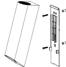
2. Slide the unit down to its backplate and press against the wall to secure into place.
