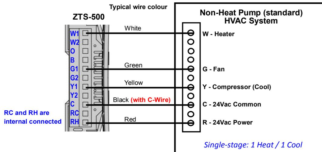
Figure 8. Non-heat pump (Standard Gas or Electric) HVAC system wiring
