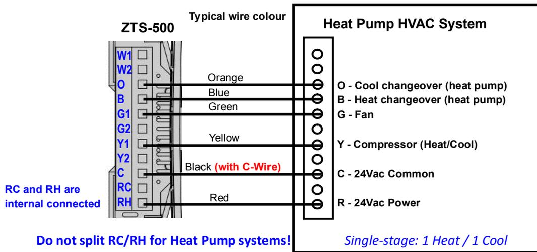
Figure 11. Heat pump HVAC system wiring
