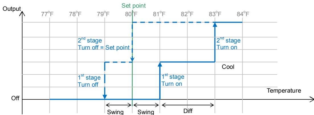
**AUTO mode:** Thermostat controls the temperature according to the following diagram.
