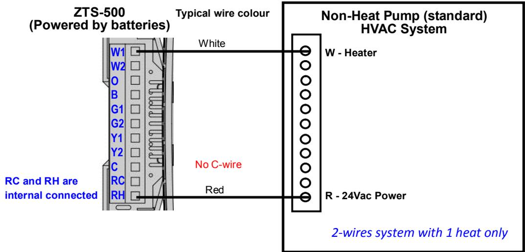
Figure 9. Non-heat pump (Standard Gas or Electric) 2-wires HVAC system wiring
