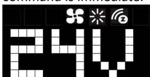
If it is powered by 24Vac or 24Vac plus batteries, ZTS-500 will self-configure to Always Listening Mode.
