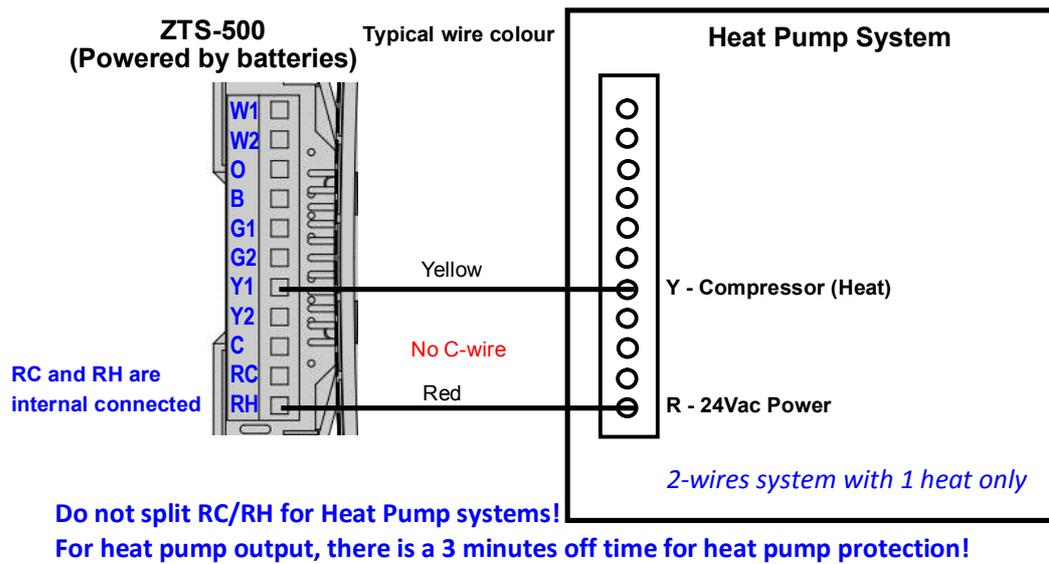
Figure 12. Heat pump 2-wires HVAC system wiring
