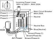
To perform the electrical installation for your Home Energy Meter (HEM), utilize the previous images to determine the phase version of the HEM and to also illustrate the following steps 3 through 7.
