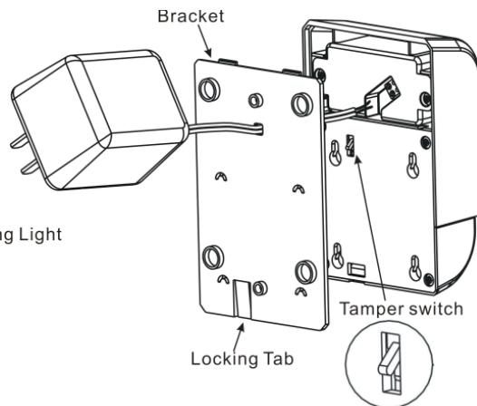
**NOTE:** This unit must be "included in the Network" **only where it will be permanently installed**. The proper operation of this node in the mesh network is dependent on it knowing its location with respect to other nodes. You cannot "test bench" configure this module, then install.
