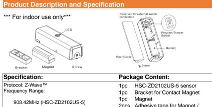
Operating Range: Up to 100 feet line of sight Operating Temp.: -15°C~ 60°C (5°F ~140°F) Battery: Panasonic CR123A \* 1PC
