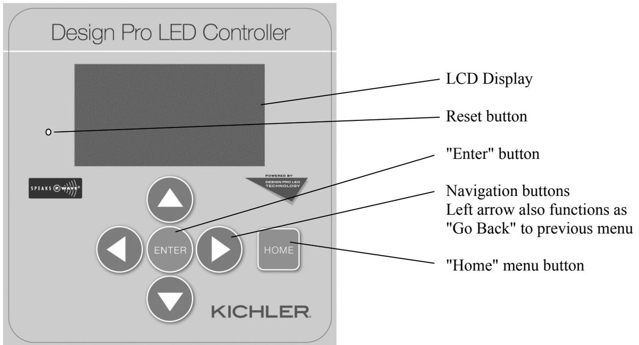
LCD Display – Graphical interface for user input and feedback
