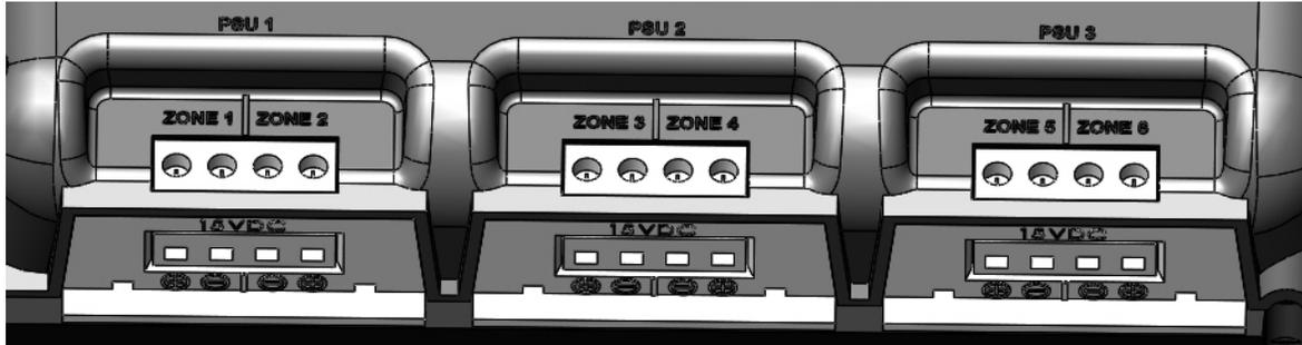
Each zone is also capable of having multiple wire runs provided the 100 Watt per PSU limit is not exceeded. Use wattage value (not VA) provided for each fixture to calculate the load on the Controller. There are no minimum load or polarity requirements for loading the Controller.
