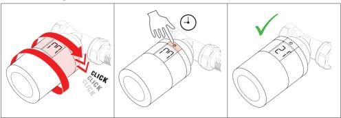
Screw the Danfoss  $Eco^{TM}$  onto the mounted adapter until a click sound appears. Once the thermostat is tightened properly, then adjust the display to your preferred display orientation. A large  $\mathfrak{M}$  is flashing in the display to indicate that Installation Mode is activated. Press and hold the button  $\overset{\textcircled{}}{}$  for 3 seconds.
