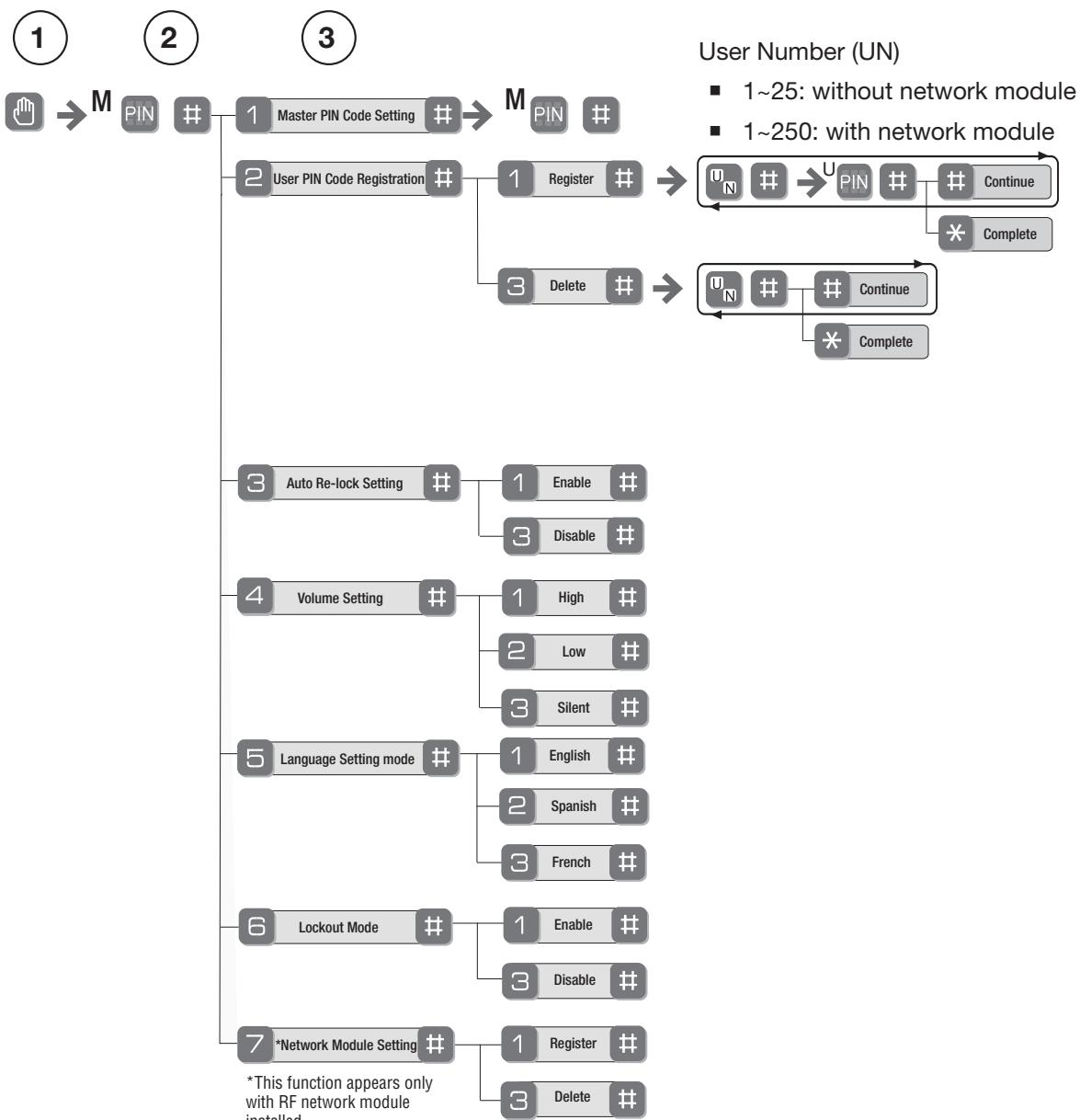
CAUTION: When joining a network your controller may or may not be aware of any previously saved user codes stored in the lock. It is recommended that all user codes be deleted from the lock prior to joining a network.
