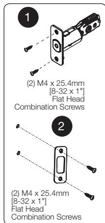
2. Install strike on the door frame, making sure to allow for the bolt to be centered in the strike.
