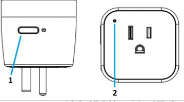
1. On/Off and Pairing Button 2. On/Off , Pairing and alarm LED (Green)
