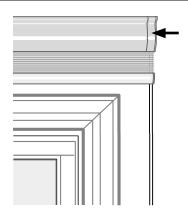
1. Press and hold the button on the headrail endcap until the shade jogs twice (about 15 seconds), then release the button.
