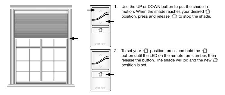
**Note:** Always adjust the upper and lower limits before adjusting your position. After adjusting the upper or lower limits, the position will reset to the new mid-legnth position.
