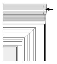
1. Press and hold the button on the headrail endcap until the shade jogs once (about 7 seconds), then release the button.
