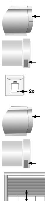
1. Press and hold the program button on the headrail/motor end, the LED will flash green then amber. When the shade jogs once, release the button and the LED will turn solid amber and turn off. The motor is now ready to learn a new remote.
