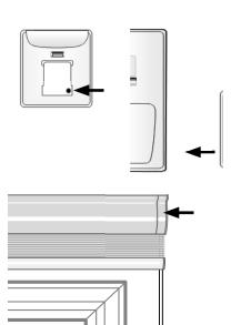
Press and hold the programming button until the LEDs stop blinking. LEDs will blink green, amber, red, and then finally turn off (about 15 seconds).
