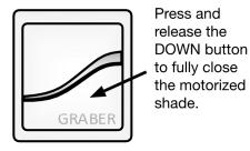
Note: you can press and release the opposite directional button to stop the shade while it is in motion.
