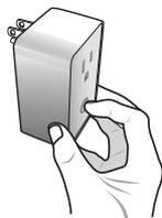
3. Plug the PA-100 back into the AC outlet with the button pressed
