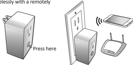
A Z-Wave certified controller is capable of setting up ZLINK products in your desired network. Once the device is added, you may assign it to a Group. Furthermore, it can be set in Association with another Z-Wave device to perform a specific triggered function such as turning lights on when motion is detected. Please refer to the instructions manual of your controller for details and procedures on how these settings can be done.
