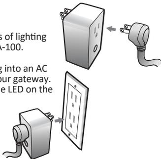
**Step 2** Insert the module's 3-pin plug into an AC outlet in the same room as your gateway. In normal operating mode, the LED on the front panel will be lit.
