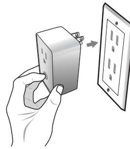
After 3 seconds, release the button. If you see the button blink, that means that PA-100 has been reset successfully and you may retry Step 3 above to add the module into your network. Otherwise, please repeat the manual reset procedure.
