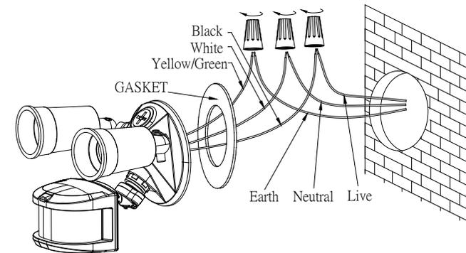
3. Disconnect the mains wire from the floodlight by untwisting the wire nuts.
