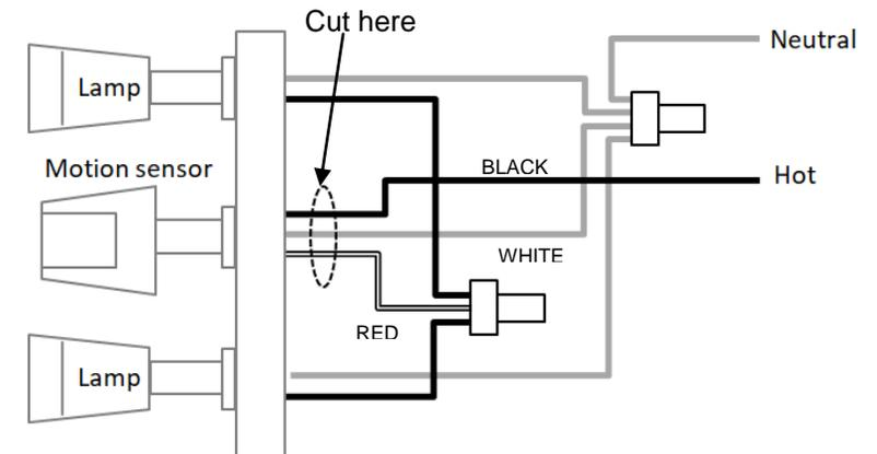
6. Disconnect the wires of the motion sensor by cutting it if necessary.
