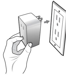
After 3 seconds, release the button. If you see the button blink, that means that PD-100 has been reset successfully and you may retry Step 3 above to add the module into your network. Otherwise, please repeat the manual reset procedure.
