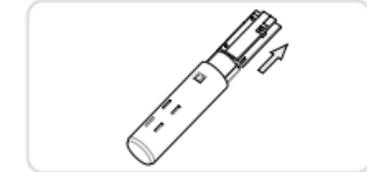
3. Remove the clear battery insulator by pulling it away from the Main Sensor.
