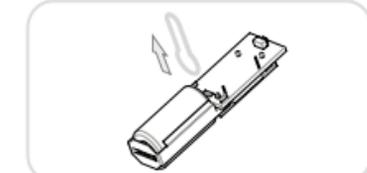
4. With the battery insulator removed, reinsert the internal components into the Main Sensor's enclosure before reattaching its lid. Ensure that the Main Sensor's button aligns with the button hole of its lid. The Main Sensor will now look as it did prior to step 1.
