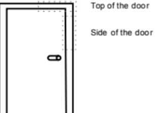
The rectangular areas highlighted above are optimal installation positions.
