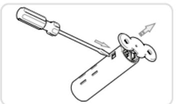
2. Separate the Main Sensor's two sections by first removing its lid and then removing its internal components.
