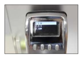
2) **1:N** - When this is chosen, all users enrolled at this lock only need to match their enrolled Fingerprint OR PIN Code to unlock the door.
