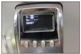
8) With the cursor on the "From" hour, use the Up/Down arrows until desired hour is shown. Press **M** to save selection.
