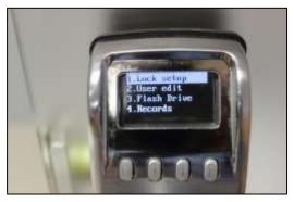
The Lock Setup menu will then automatically display the Lock Menus: Note: Lock menus 1 through 4 are displayed. Press the Down arrow button to view menus 5-6.
