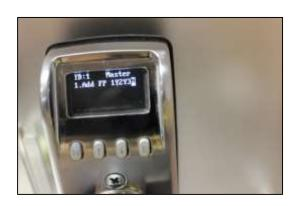
9) Rest finger on sensor. Press the Up Arrow to highlight "3N." Press **M**.
