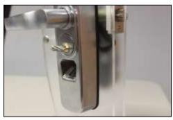
2) Turn the key in a clockwise direction to horizontal level (90 degrees).
