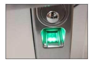
2) After the fingerprint sensor illuminates, rest the enrolled finger on the sensor window to verify.
