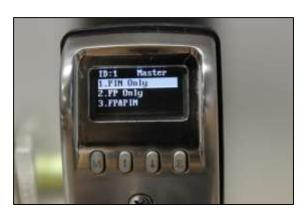
This menu will be displayed. It allows deletion of "PIN Only", "FP Only", or both "FP&PIN".
