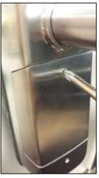
1) Remove the battery cover of the inside unit by removing the screw shown. This will make installing the inside unit an easier process.
