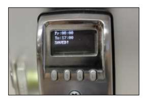
10) After the desired Time Frame has been selected, press **M**. Message "SAVED?" will display on the LCD.
