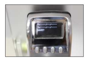
3) The "From" and "To" Date Range options will be displayed. The format for the Date Range settings is MM/DD/YYYY. Press **M**.
