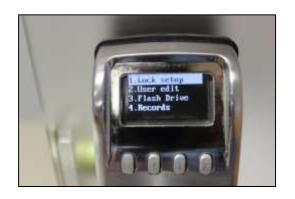
2) Option 1 "Lock setup" is highlighted. Press **M.**
