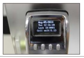
5) Press **M** on the inner keypad of your RTS to initialize the lock and display the current battery voltage.
