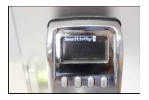
2) Use the Up/Down arrows to scroll thru the sensitivity levels until the desired level is reached. Press **M**.
