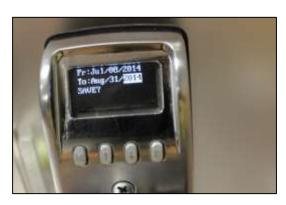
4) Use the Up/Down arrow keys to choose the DD & YYYY. When desired value is chosen for each section, press **M** to move to the next value.
