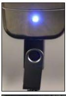
1) Insert USB thumb drive in the inside unit located at the bottom of the lock.
