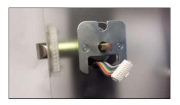
1) Insert the Spindle though the fixing plate and into the inside section of the lock's spindle hole.
