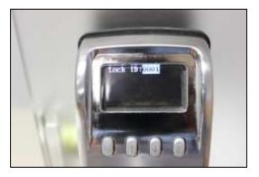
2) Use the Up/Down arrows to scroll to the desired lock ID. Press **M** to save setting.
