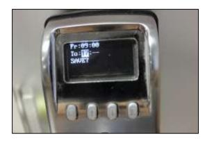
9) With the cursor on the "To" hour, use the Up/Down arrows until desired hour is shown. Press **M** to save selection.
