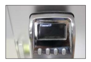
After the Lock Menus are dis-played, if no buttons are pressed for 17 seconds an audible alert (2 beeps) will be heard and then a "Timeout!" message will be dis-played. The lock will then shut down. The setup process can be started again by pressing any of the 4 buttons on the lock front.
