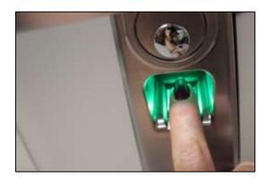
3) If fingerprint verification is successful, a single short beep will be heard, the green LED will flash and the RTS will unlock. It will remain unlocked for approximately four seconds.
