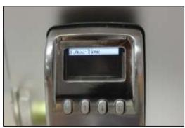
3) **Acc-Time** (Access Time) - This mode allows for timed access to the lock to be created for a specific date range, days of the week and time frame within the days of the week.
