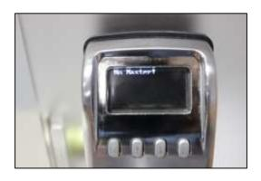
**No Master!** Screen indicates that no fingerprints or User PINs have been programmed into the lock.
