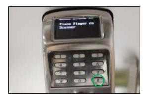
1) Enter the User ID on the key-pad of the outside unit. Then press the # button. The sensor will illuminate. Example: User 50 would press "50#".
