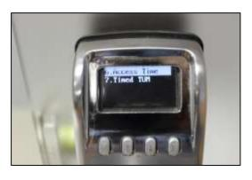
1) In the Lock setup menu, scroll to Option 6 "Access Time". Press **M**.
