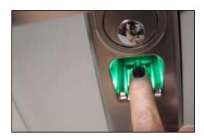
6) The sensor will flash 3 times. Keep finger on the sensor while it flashes.
