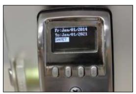
5) Once the Date Range is entered, press **E**. "SAVE?" will display on the LCD. Press **M** to save. Press **E** to exit without saving.
