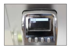
3) **1:1** – When this is chosen, all users enrolled at this lock must enter their User ID and verify their enrolled Fingerprint or PIN Code to unlock the door.
