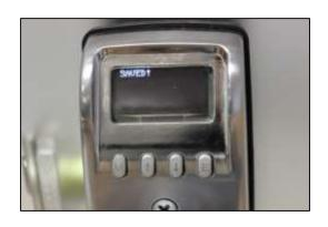
3) "SAVED!" indicates the Sensitivity level settings were saved. This will display momentarily and then the setup menu will be shown.
