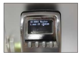
5) "Add FP" is displayed along with "1N2N3N". "1N" is highlighted. Place finger on the sensor. Press **M**.
