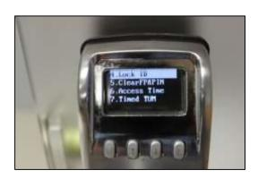
1) In the Lock Setup menu, scroll down to Option 4 "Lock ID". Press **M**.
