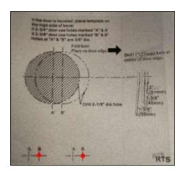
4) Move the template back to the door. Align it again and then mark the holes onto the door.
