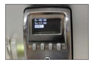
5) Once the Time Frame is set up, press **E**. "SAVE?" will display on the LCD.
