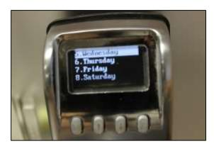
3) When completed, press **E**. "SAVE?" will display on the LCD. Press **M** to save.
