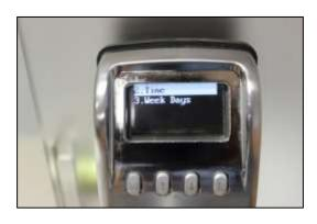
7) Scroll to "Time" and press **M**. The current setting for "From" and "To" are shown. Press **M** again.
