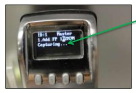
"Capturing..." will be shown while the FP is being scanned.
