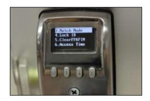
1) In the Lock setup menu, scroll down to "Match Mode" and then press **M**.
