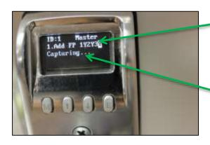
When 3 fingerprint matches for a user have been successfully enrolled, "1Y2Y3Y" will be displayed.
