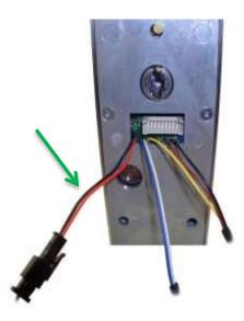
The red and black wires have a connector that can be detached and wired to a 6V power supply. Disconnect the wires and hard wire to the 6V source. Once hard wired reconnect to the lock.
