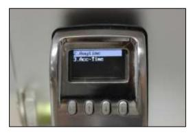
2) **Anytime** - When this is chosen, the lock allows all enrolled Users to unlock the door. The exception to this is if specific Timed Access is set up for individual Users (see Section 2: User Edit).
