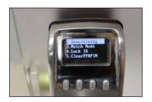
1) In the Lock setup menu, scroll to Option 2 "Sensitivity". Press **M.**
