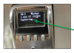
"Capturing..." will be shown while the FP is being scanned.
