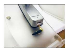
1) Take the antenna out of bag "E" and remove red plastic cover. Then screw the antenna on the bottom of the inside unit.
